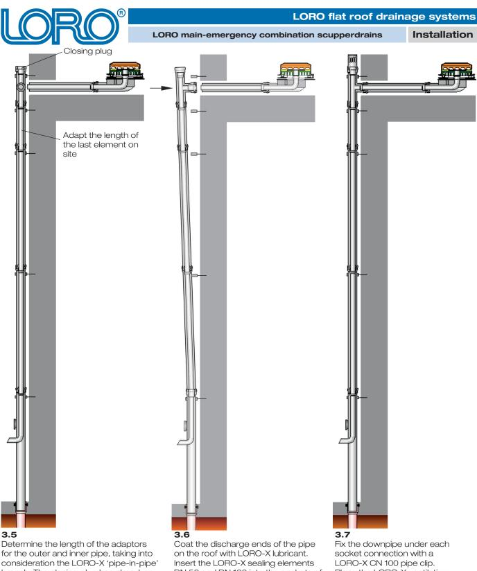
branch. The closing plug has already been fitted to the socket of the inner pipe DN 50 in the factory. Make the socket joints of adaptors and double pipe branch as described.
