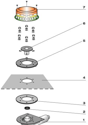
Screw the strainer to the loose flange using the 3 fastening screws provided.
